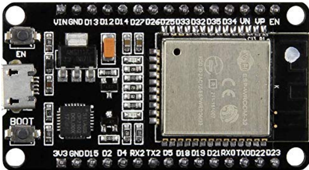
Figure 3.7 – ESP32 DEVKIT V1
